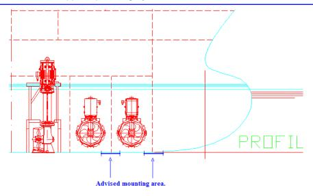
The generally best placement on larger vessels is in the front region of the vessel just behind the bulbous bow (see fig above). This area is generally designed such that the bubbles are pushed to either side of the bulb, leaving a clear area under the bulb and just behind. The sensor is installed in a sea valve in order to service the sensor (clean or replace) without docking the vessel.
