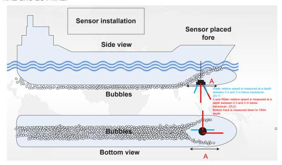
There are 2 channels in DL2. The acoustic signal is sent in a 30deg angle in forward and starboard directions.
