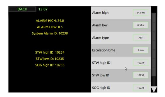
Remote acknowledge can be set up by aux input, by ACK or ACN (both from NMEA port and LAN). Alarms are available for low speed (SOG and STW), high speed(SOG and STW) and system failure. They can be activated or deactivated and given a unique alarm ID. Each alarm has its own unique ID and message, and can be deactivated by making the ID zero.
