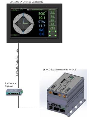
**NOTE:** The following procedure will take you through the setup using the operator unit CU-M001. It is important to change the JB70D2-SA group before the CU-M001-SA group otherwise you will loose connection
