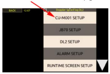
To enter and adjust these screens a password is required. The password for all units is 'service'. The password will be remebered for 1 hour, or until reboot of the system.
