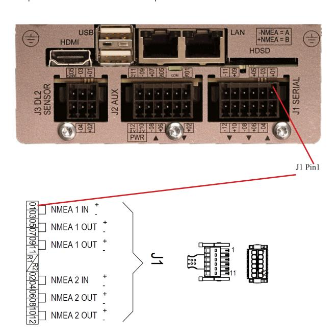
If high speed prototcols are to be used (IEC61162-2) the communication common (COM) can be connected to pins 11 or 12 of J2
