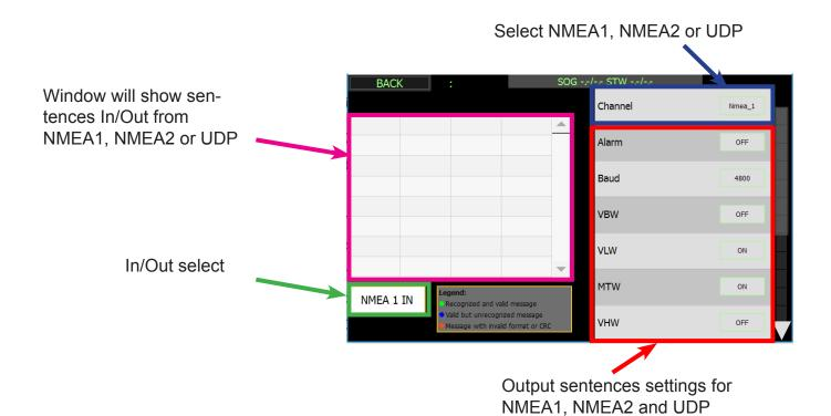
For each of the outputs 1, 2 and LAN it is possible to activate a number of sentences. Normally with On and Off. The resulting outputs are shown on the left on the screen.
